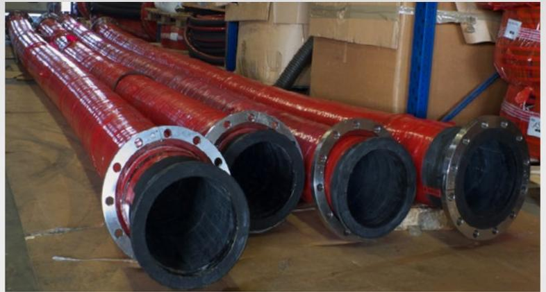
Flexibles hoses for phosphoric acids fitted 8" cam & groove couplings stainless steel 904L
