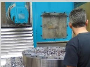
Inhouse machining of CF swivel ring
